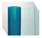
Formulated for superior flexibility in low temperature applications, our low temp clear PVC panels are the perfect solution for cold storage or food manufacturing applications down to -25 degrees. This PVC formulation is compliant with all relevant federal and international food safety standards. Panels are available in available in .275" or .354" thicknesses.
