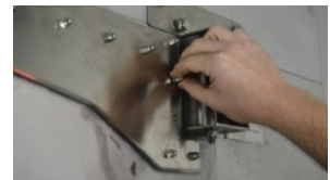
Figure 9: Adjusting tension spring
