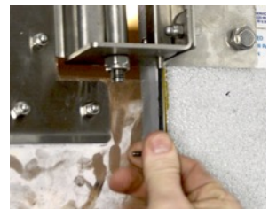
Figure 9: Adjusting tension spring
